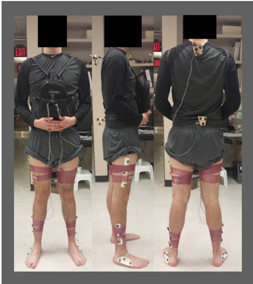
Figure 32: Anterior, lateral and posterior view of IRED placement on test subject.
