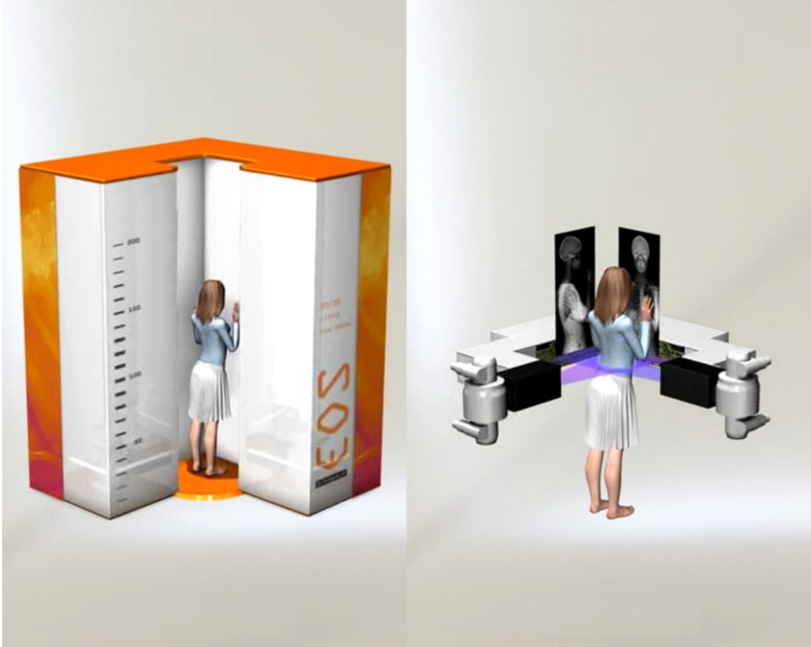
Figure 3: EOS image collection representation. Two low-dose X-ray tubes move vertically, simultaneously capturing biplanar digital images of patient. Radiation beams produce 45cm wide scanning area, resulting in rapid, high quality images with pronounced accuracy and little to no error resulting from source-to-plate angles [30].
